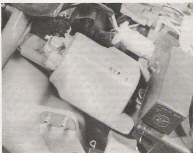
7.1 Ignition coil is bolted to frame below the fuel tank
