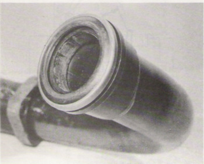
10.6 Use new exhaust port seals to prevent gas leakage
